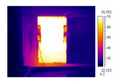
**Phase change cooling system** Higher thermal conductivity Swifter heat diffusion, subtle temperature deviation Even heat distribution on housing The whole shell as heat sink, less weight and cost
