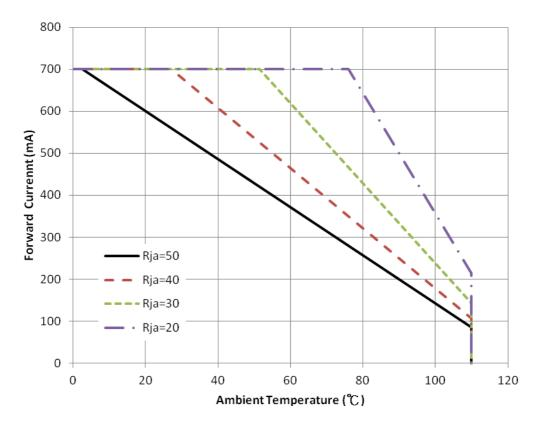
The junction temperature can be correlated to the thermal resistance between the junction and ambient (Rja) by the following equation.
